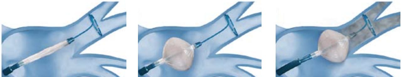
A graphic illustration of cryo balloon ablation using the Arctic Front cryoablation catheter
